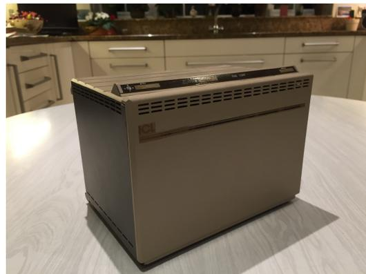
Rob Wilmott had been appointed Chief Executive of ICL and wanted a small office computer running the VME operating system, with the power of a mainframe but requiring no false floor, fan or air conditioning. It had to be capable of operating as a dual node system, use the fast fibre optic macrolan for disks and slower OSLAN for other peripherals.
